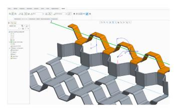
Create sheetmetal geometry using functionality to automatically apply bend relief, create sheetmetal rips, bend coplanar geometry, and more.
