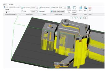
Position the model on the print tray and view the required supporting material in Creo.
